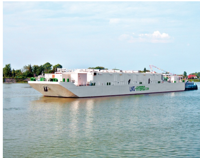
Hybrid power barge
